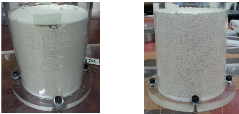
(a) Sample 1 - Double-porosity soil (25% m/c) (b) Sample 2 - Double-porosity soil (30% m/c)
