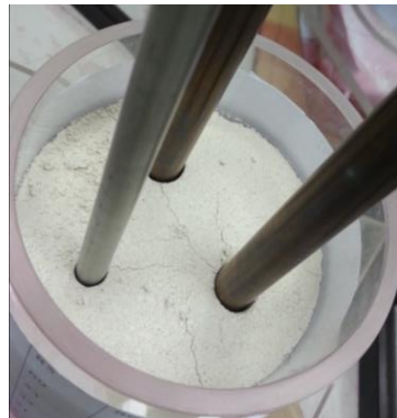
Fig. 4. Fractured double-porosity soil sample after vibration is applied
