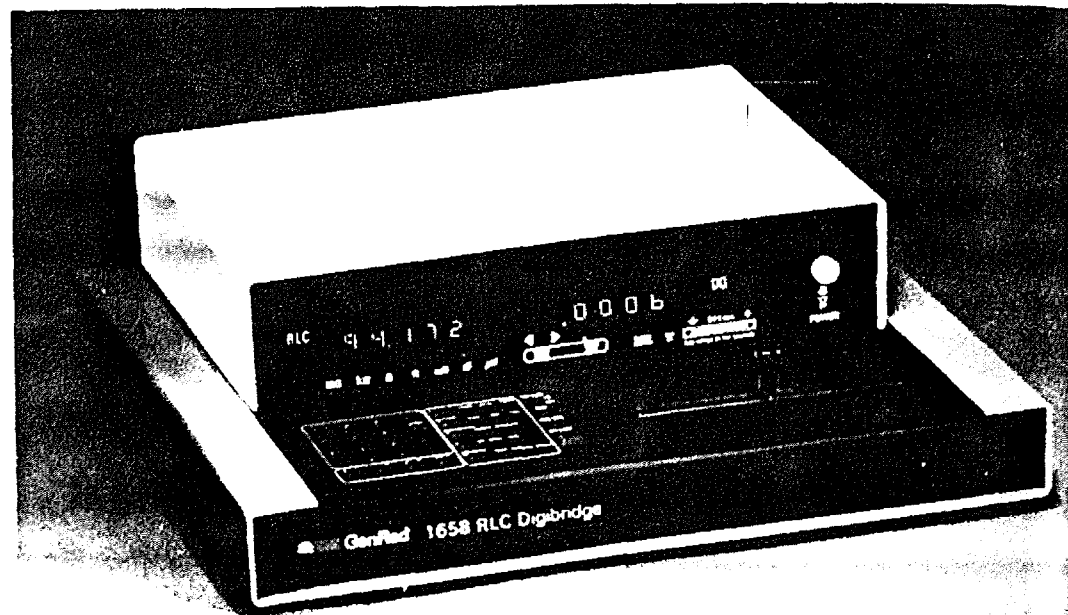
FIGURE 5-14 General Radio, Model 1658 RLC Digibridge. (Courtesy GenRad Inc., Concord, Mass.)
