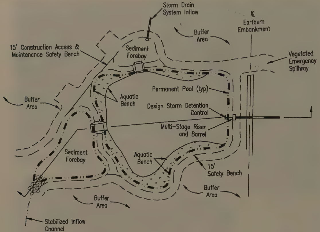
Figure 14.7 Wet Stormwater Retention Pond with Earthen Embankment. Schematic shows different pool heights for different storage levels. Source: State of New York (2001).
