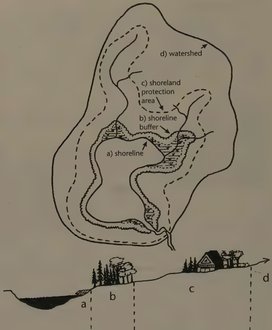
Figure 14.2 Four Zones of Lake Protection. Source: Karen Cappiella and Tom Schueler, 2001, "Crafting a Lake Protection Ordinance." Reprinted courtesy of the Center for Watershed Protection.
