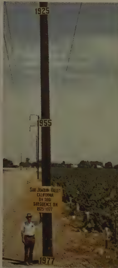
Figure 9.22 Ground Level Drop Due to Subsidence from Groundwater Withdrawal in San Joaquin Valley, California, Near Mendota. Approximate altitude of land surface based on research efforts of Joseph F. Poland (pictured). Source: U.S. Geological Survey (2000c).
