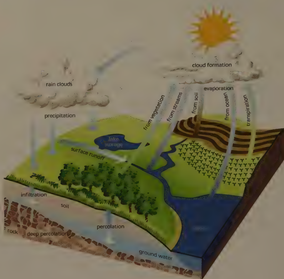
Figure 13.1 Hydrologic Cycle. The transfer of water from precipitation to surface water and groundwater, to storage and runoff, and eventually back to the atmosphere is an ongoing cycle. Source: FISRWG (1998).
