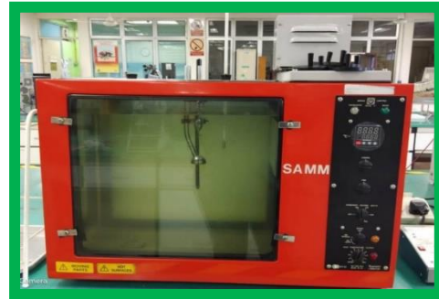
Kinematics Viscosity Townson+Mercer Viscometer
