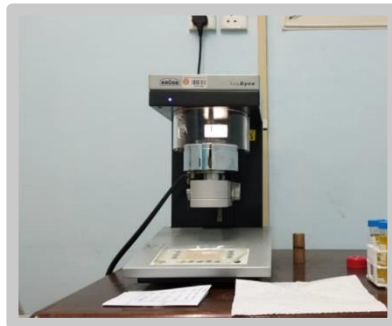
Surface Tension Kruss Tensionmeter
