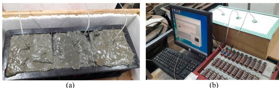
Fig. 3. Hydration test (a) thermocouple inserted in fresh concrete (b) test setup.
