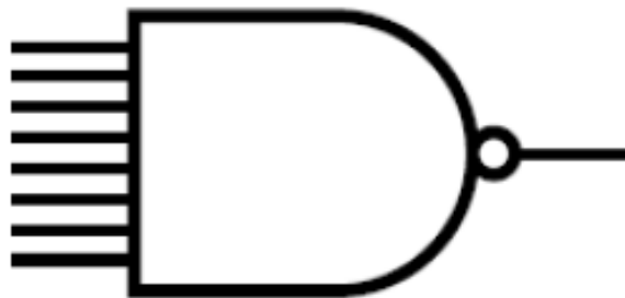
NAND gate with a fan-in of 8
