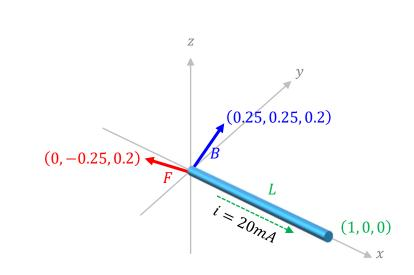
When a wire of length L carries a current i through a magnetic field B, the magnetic force |F| by the field on the wire is:
