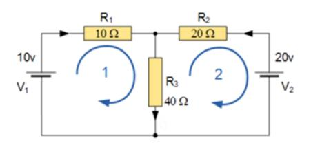
In analysing the above circuit, current on loop 1 and loop 2 can be computed based on two equation:
