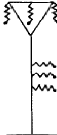
Combined 3 wire 11 kV and 380 V
