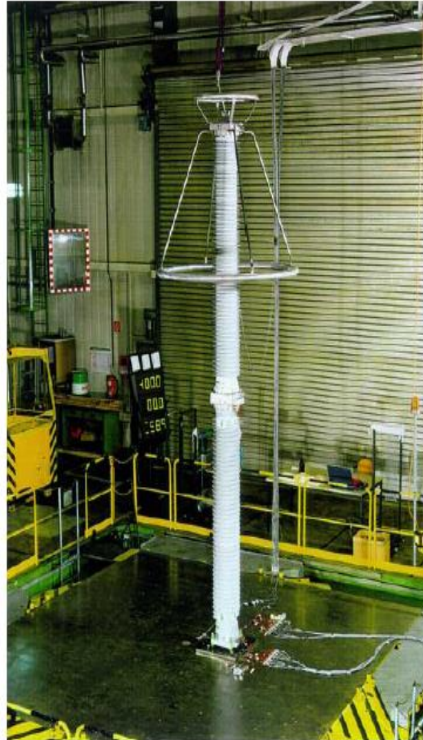
Fig. 21: Polymer housed arrester for a 550-kV-system during seismic testing on a shaking table
