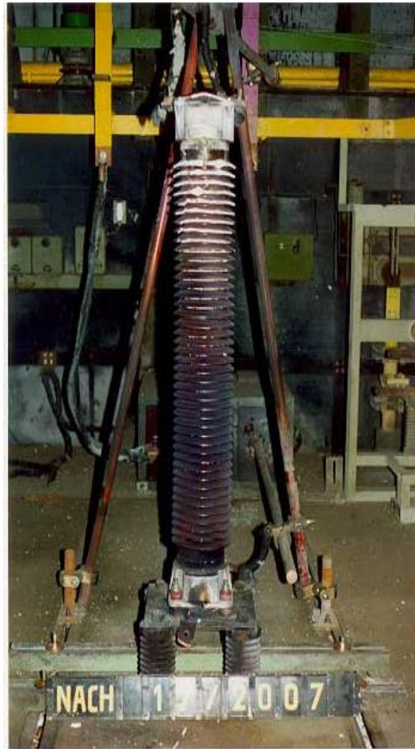
Fig. 22: Porcelain housed arrester after pressure relief test with rated short-circuit current (63 kA, 200 ms). With the exception of some sheds which were broken the housing remained intact.
