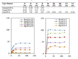
Fig. 4 Adsorption capacity of a) MVA-untreated and b) MVA-treated on multimetal adsorption (Pb, Zn, Cd, Cu, Hg)
