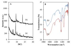
Fig. 2 A) XRD pattern and B) FTIR spectra of (a) untreated MVA and (b) treated MVA
