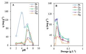
Fig. 5 Effect of A) pH and B) adsorbent dosage on the adsorption of multimetal ions onto treated MVA.
