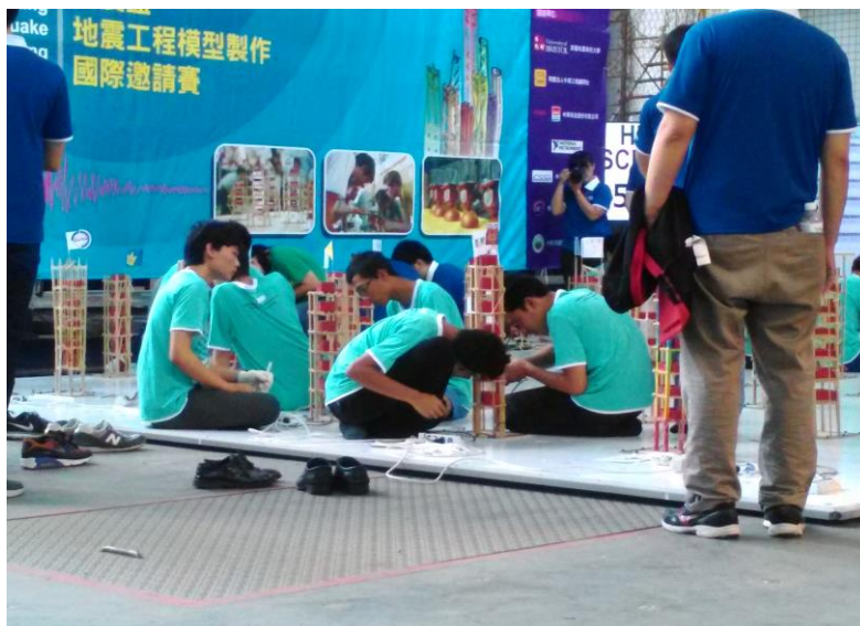
Figure 4: Participants glued loads on building and attached the building on shaking table
