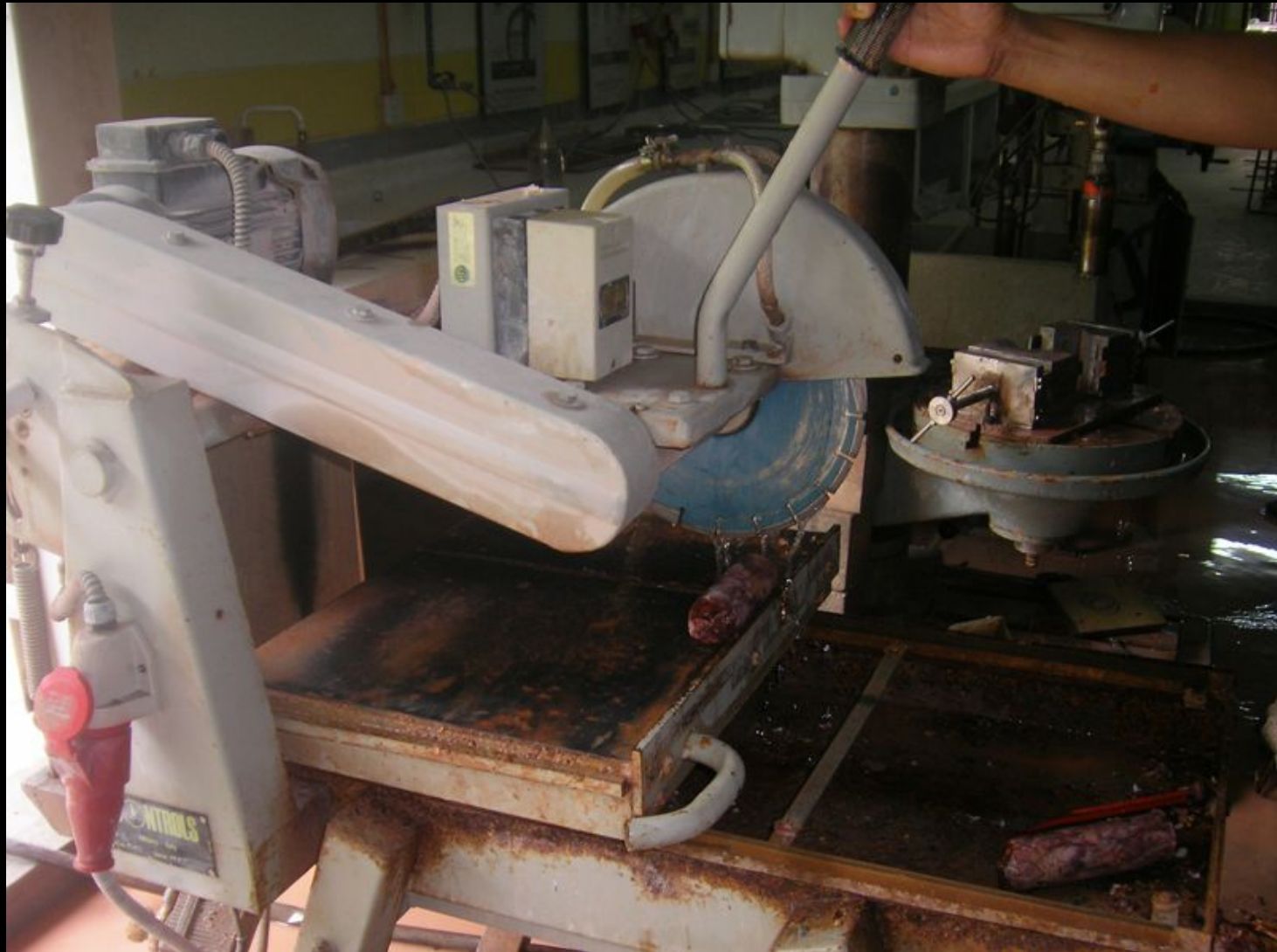
Trimming of core sample to the required height or length using diamond disc cutter.
