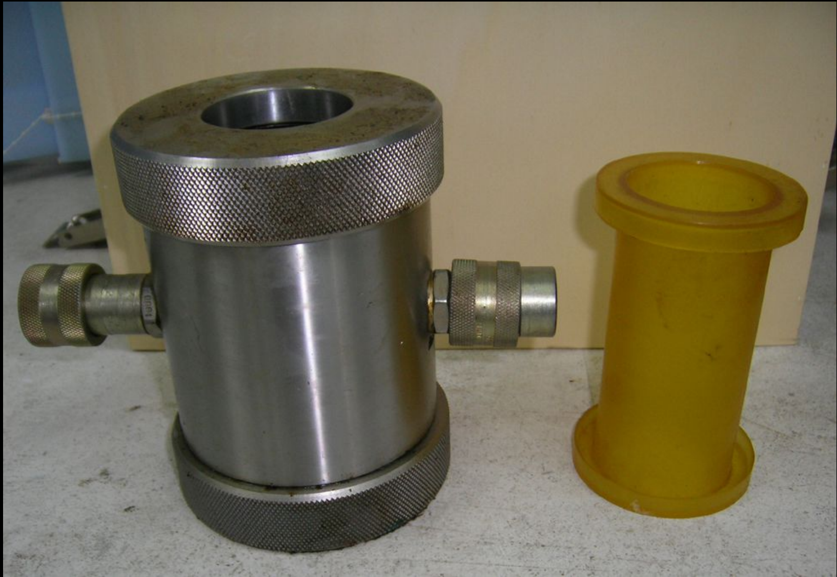
Hoek's Cell & sample sleeve for triaxial compression test on core sample of 54 mm D & 108 mm H
