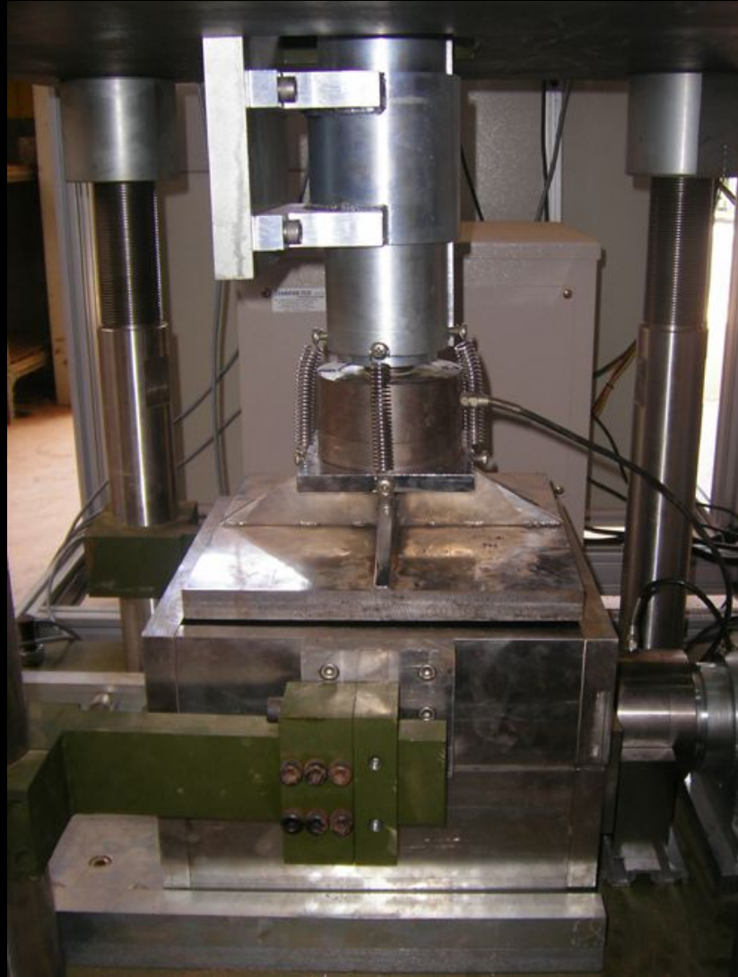
Shear box section for rectangular sample size 150 \times 220 \times 220 mm (H \times L \times B)
