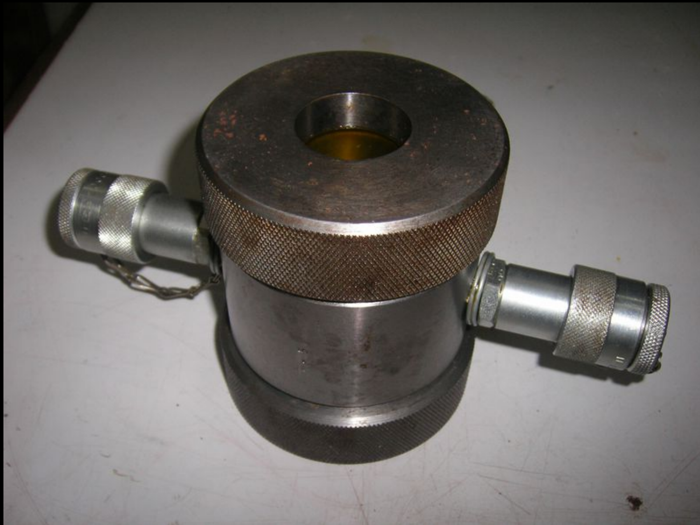
Hoek's Cell for use in triaxial compression test
