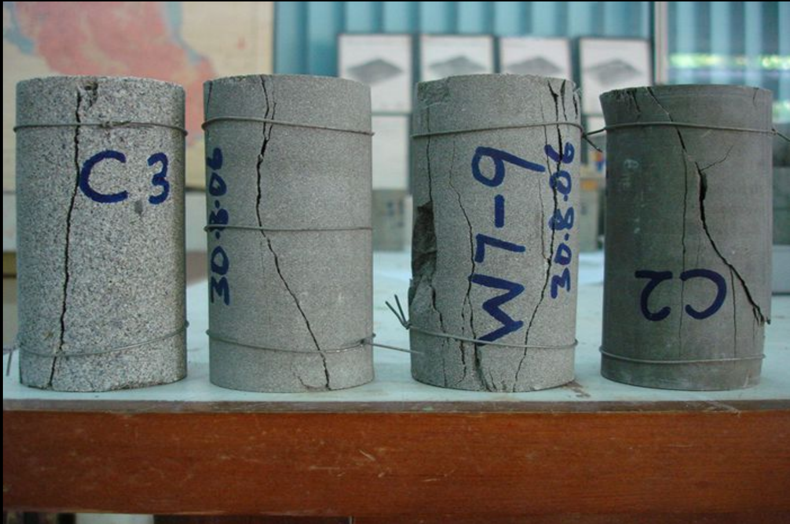
Fracture planes in failed rock sample (UCT)
