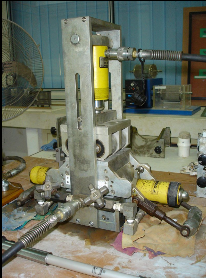
Portable shear box apparatus suitable for test on core sample (Roctest Phi – 10)
