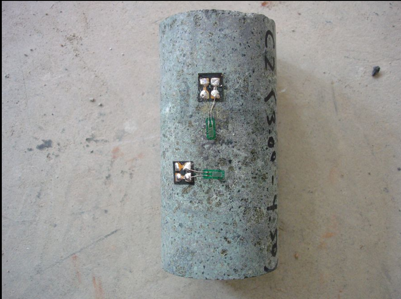
Electric foil strain gauges (20 - 30 mm gauge length) to measure strains
