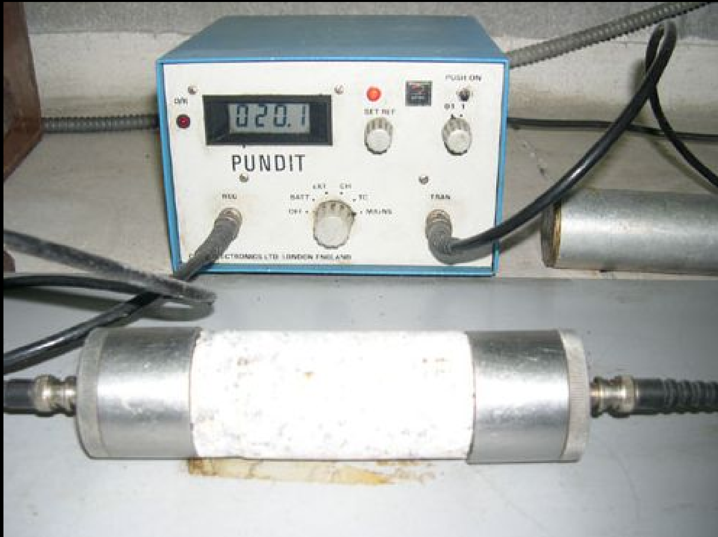
Sonic velocity test on core sample (non-destructive test, sample can be used for other test)
