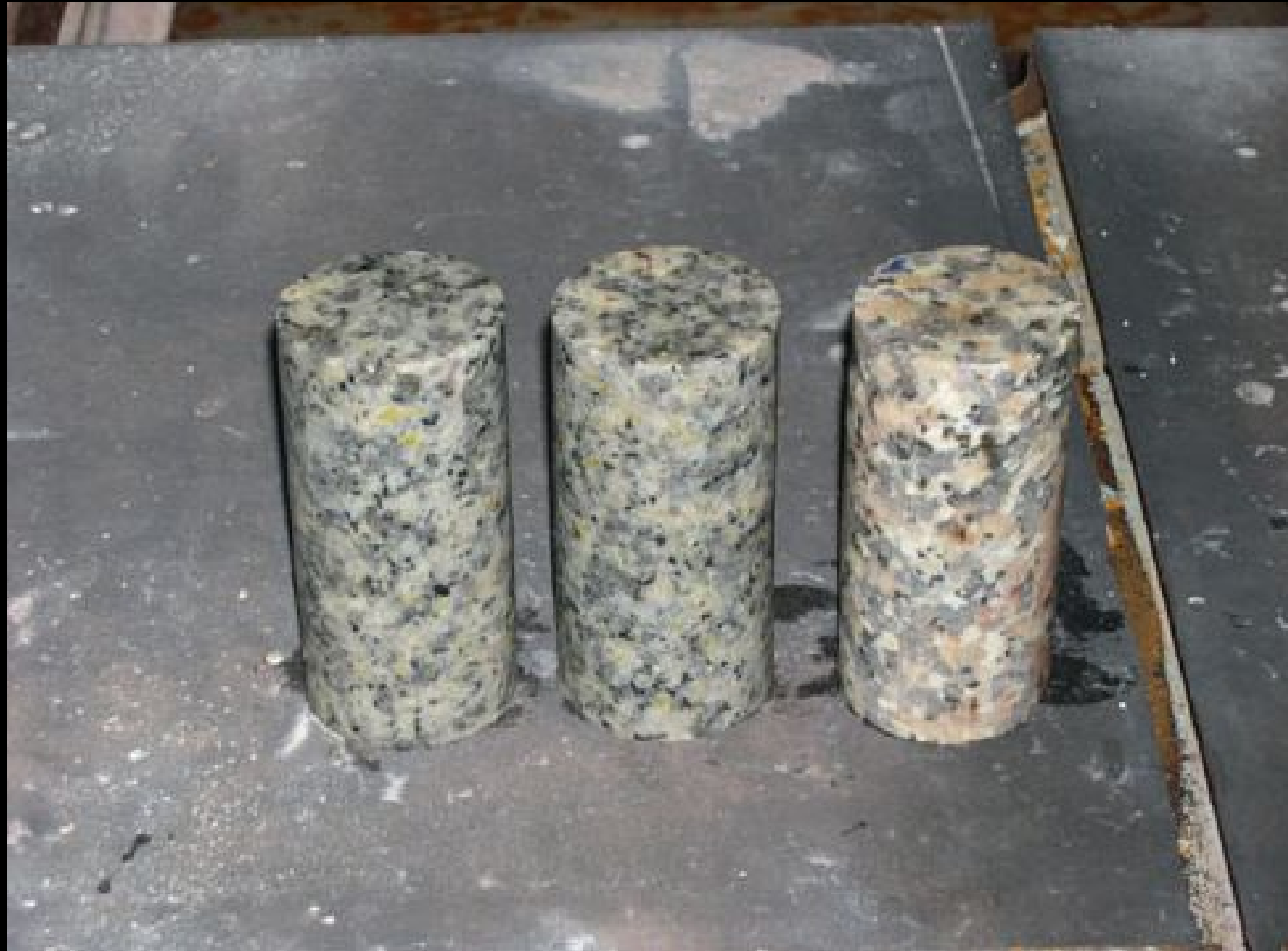
Prepared core samples – 54mm dia. & 108mm height.
