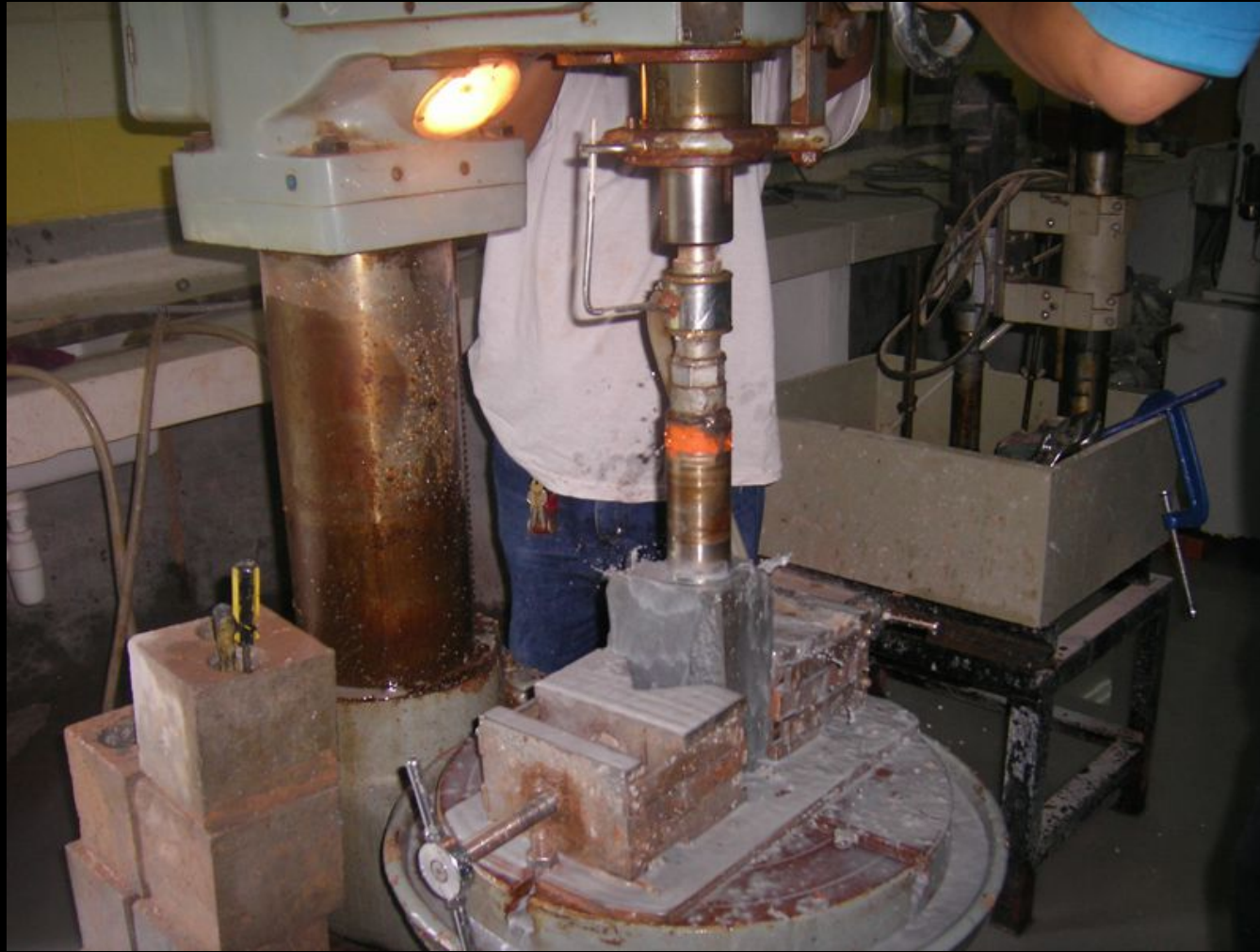
Coring of rock block in laboratory – to obtain cylindrical sample 54 mm diameter & 108 mm height
