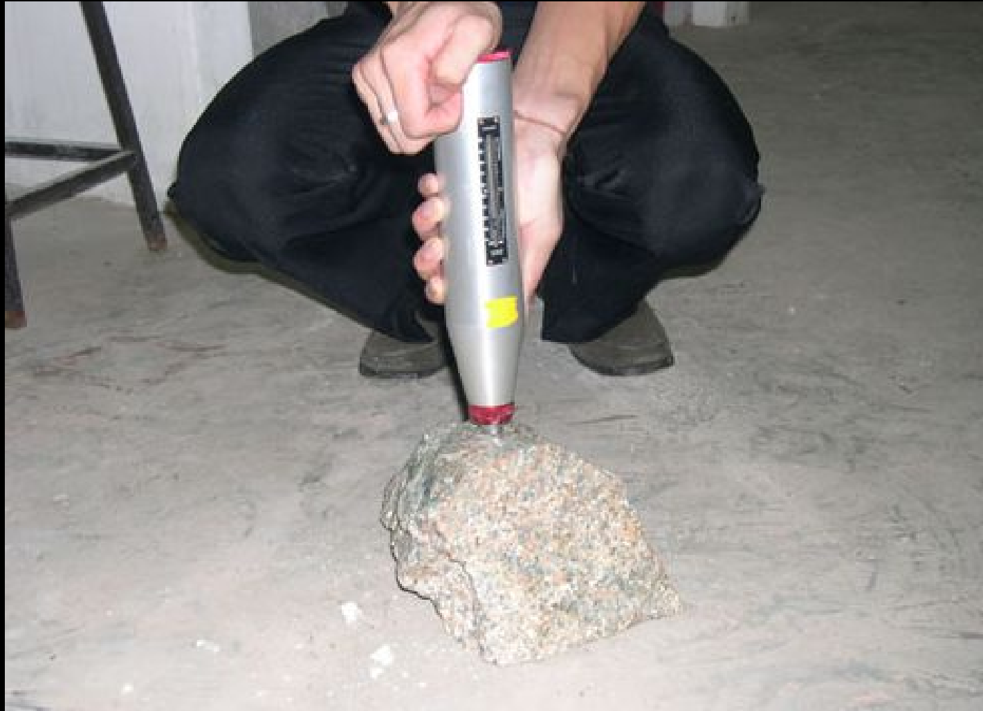
Schmidt hammer test on irregular block sample
