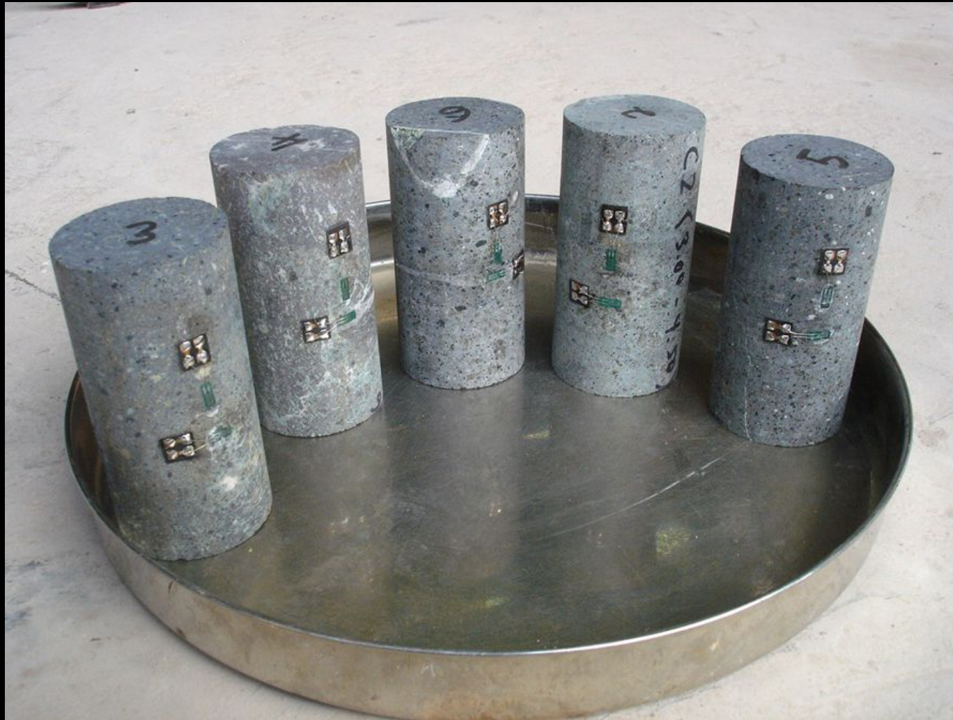
Core samples for UCS test with axial (vertical) and radial (horizontal) strain measurements
