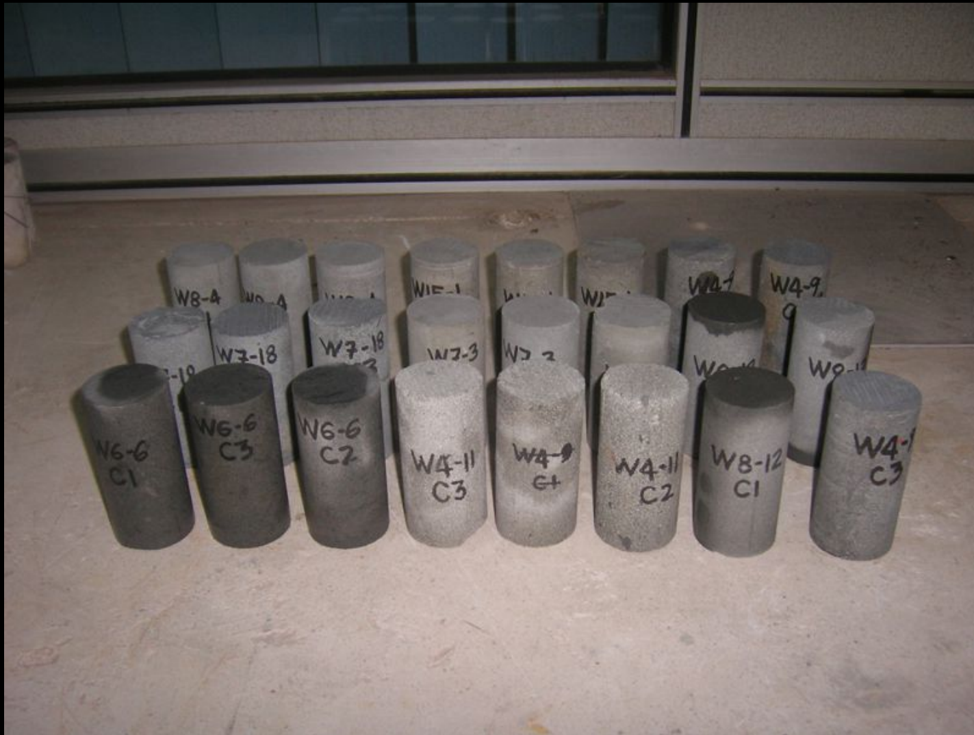
Prepared core samples – 54mm dia. & 108mm ht.
