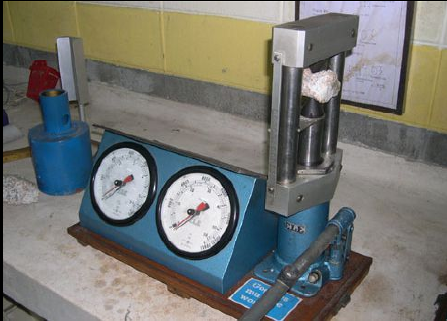
Point-load test on irregular block sample
