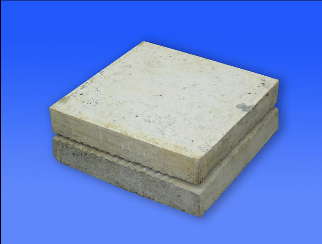
Sample of rectangular joint size 150 \times 220 \times 220 mm (H \times L \times B)
