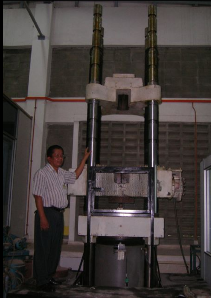
Universal compression machine, equipped with closed-circuit servo-controlled unit (3000 kN capacity)
