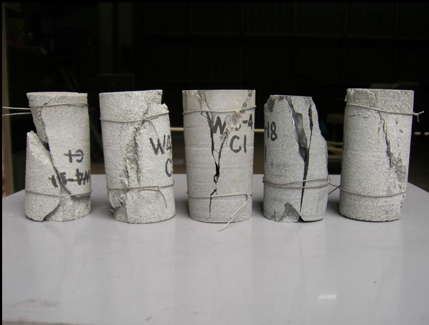
Fracture planes in failed rock sample
