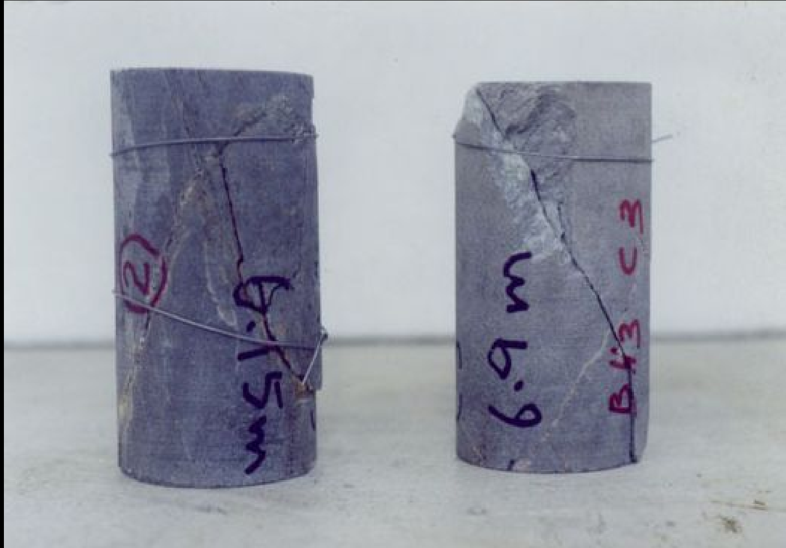
Fracture planes in failed rock sample
