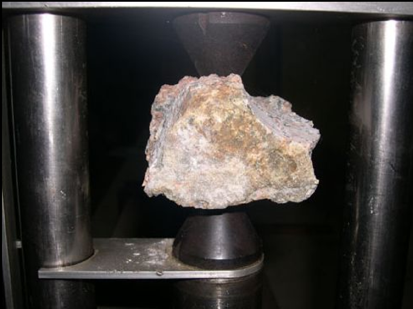
Irregular block sample placed in between pointed loading platens
