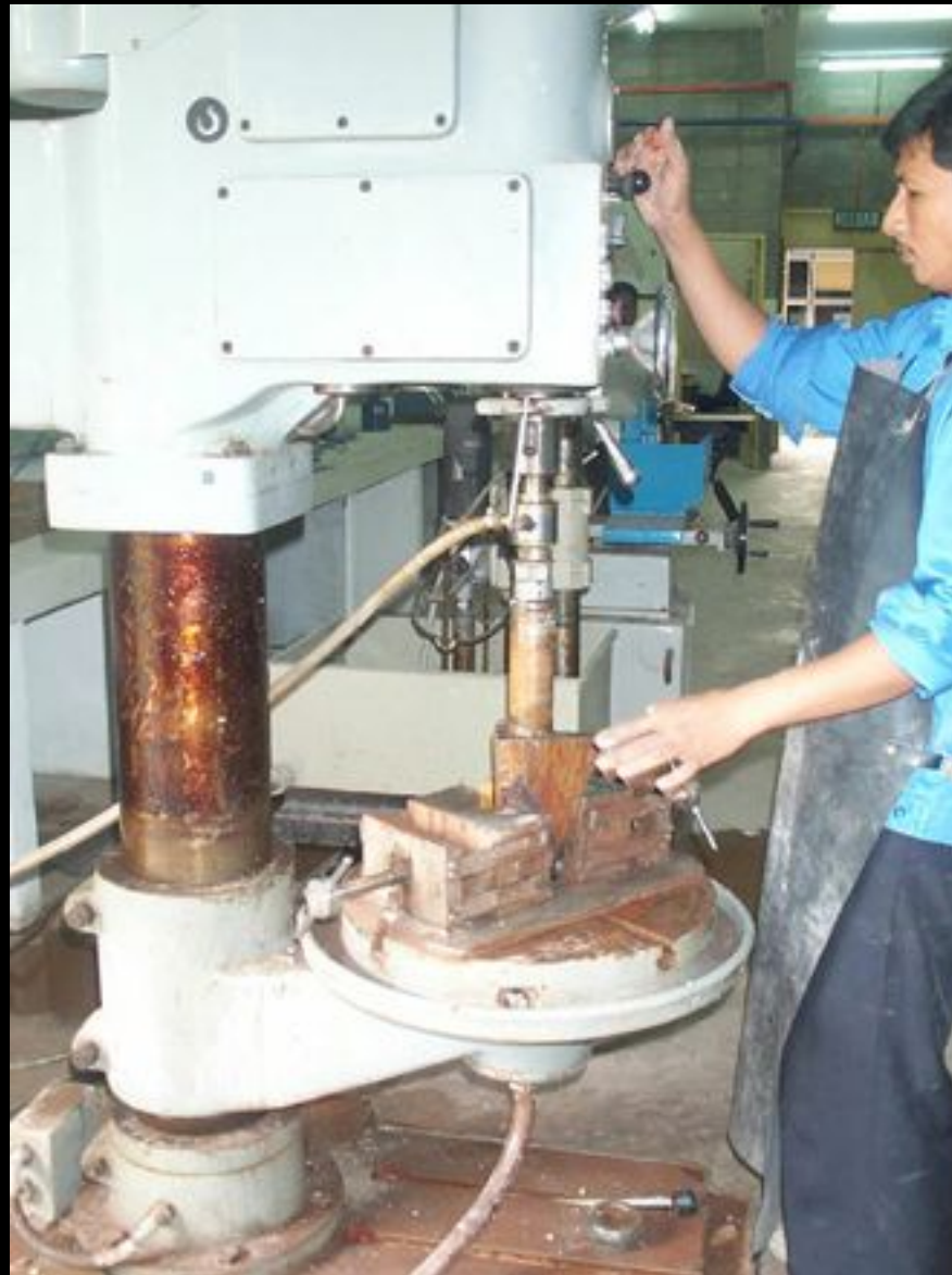
Preparation of rock core sample using laboratory coring machine (tungsten carbide coring bit)
