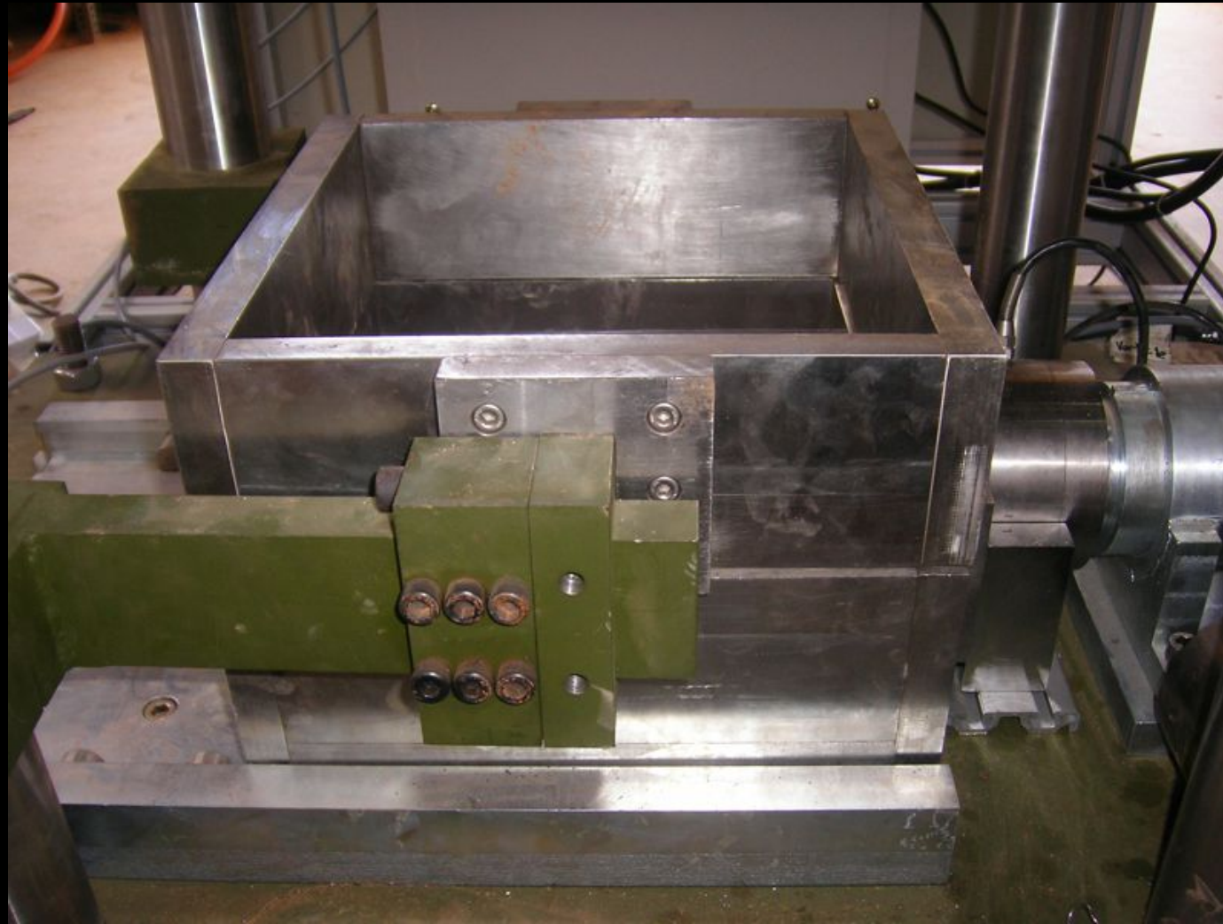
Shear box section for rectangular sample size 150 × 220 × 220 mm (H × L × B)
