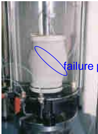
soil sample at failure
