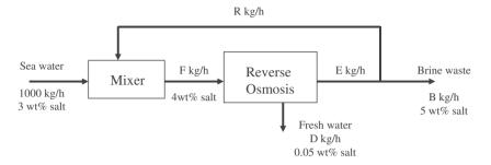
Calculate the unknown mass flow rates and the value of R/E.
