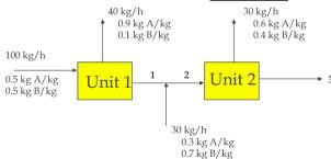
Calculate the unknown flow rates and composition of streams 1, 2 and 3
