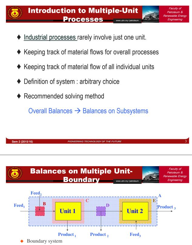
• System (overall balance) ...... Boundary A (3 inputs, 3 outputs)
