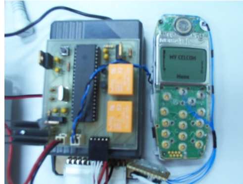
Vehicle Security System via SMS (VSSS)
