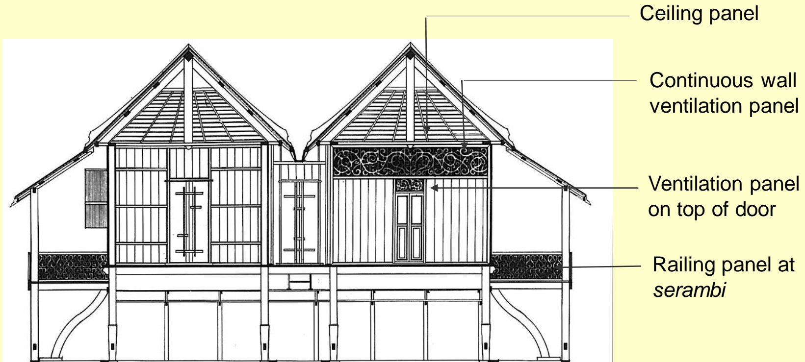
Figure 4: Railing at serambi and cared ventilation panels fitted above the interior wall of Abdul Rahim's house
