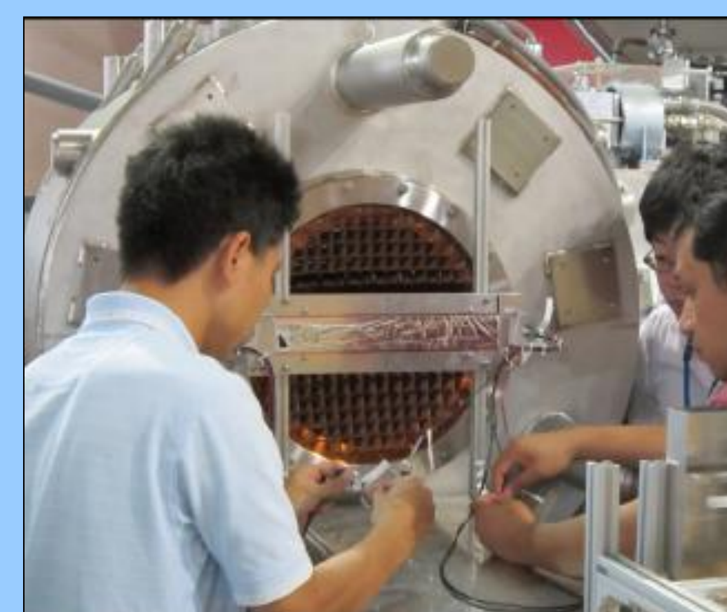
Figure 4(a): Experimental setup for muon lifetime and muonic X-ray measurements.
