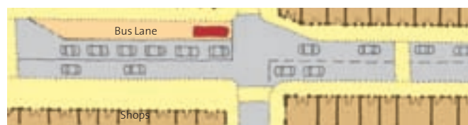
After: Reducing the number of lanes and dedicating some of the road-space as a bus lane and a widened footway enlivens the western end of the street and ensures pedestrian and public transport priority.
