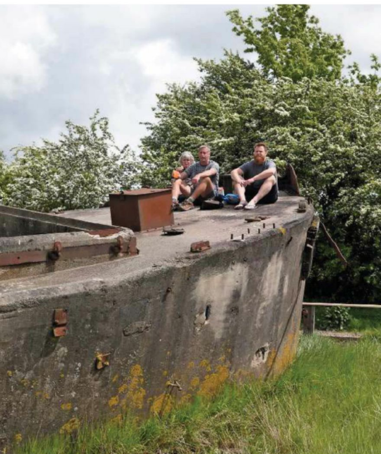
The enduring ferro-concrete barges, born out of necessity during the Second World War.
