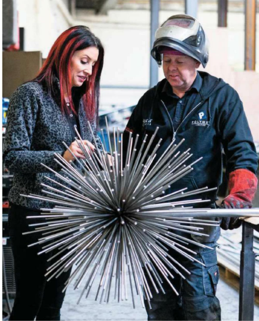
Stems are welded onto a central core, making sure they are spaced correctly. Some have different lengths and finishes that can create an interesting light effect.
