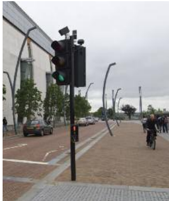
Courtesy and controlled crossings: The scheme's single Puffin crossing caused Hamilton Baillie several sleepless nights: 'Having a green traffic light facing drivers as they enter Elwick Square 'scared the hell out of me,' he says. 'I'm glad to say that it doesn't seem to have unduly damaged the scheme'. Courtesy crossings, unlike controlled crossings, have no legal status, but simply act as a guide for the pedestrian. Feedback indicates that, for drivers and the public, there is some confusion between the two, and the IDT is monitoring both types of crossings to see how they perform over time. Groups representing the blind, disabled and visually impaired would like to see more controlled crossings and more controls
