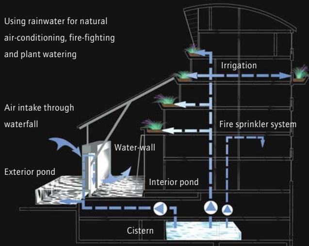
Rainwater concept with collection, storage, purification and infiltration
