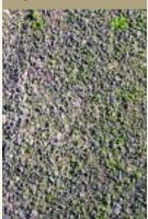
Concrete is a mix of Portland cement, sand, and aggregate (gravel). Portland cement is created in an energy-intensive process, in which clay and limestone are mixed and heated to nearly 2700 degrees Fahrenheit, releasing large amounts of carbon dioxide (a greenhouse gas) along with toxic substances such as mercury, lead, and arsenic. Cement, activated by water, binds the concrete mix together, creating a longlasting surface.
