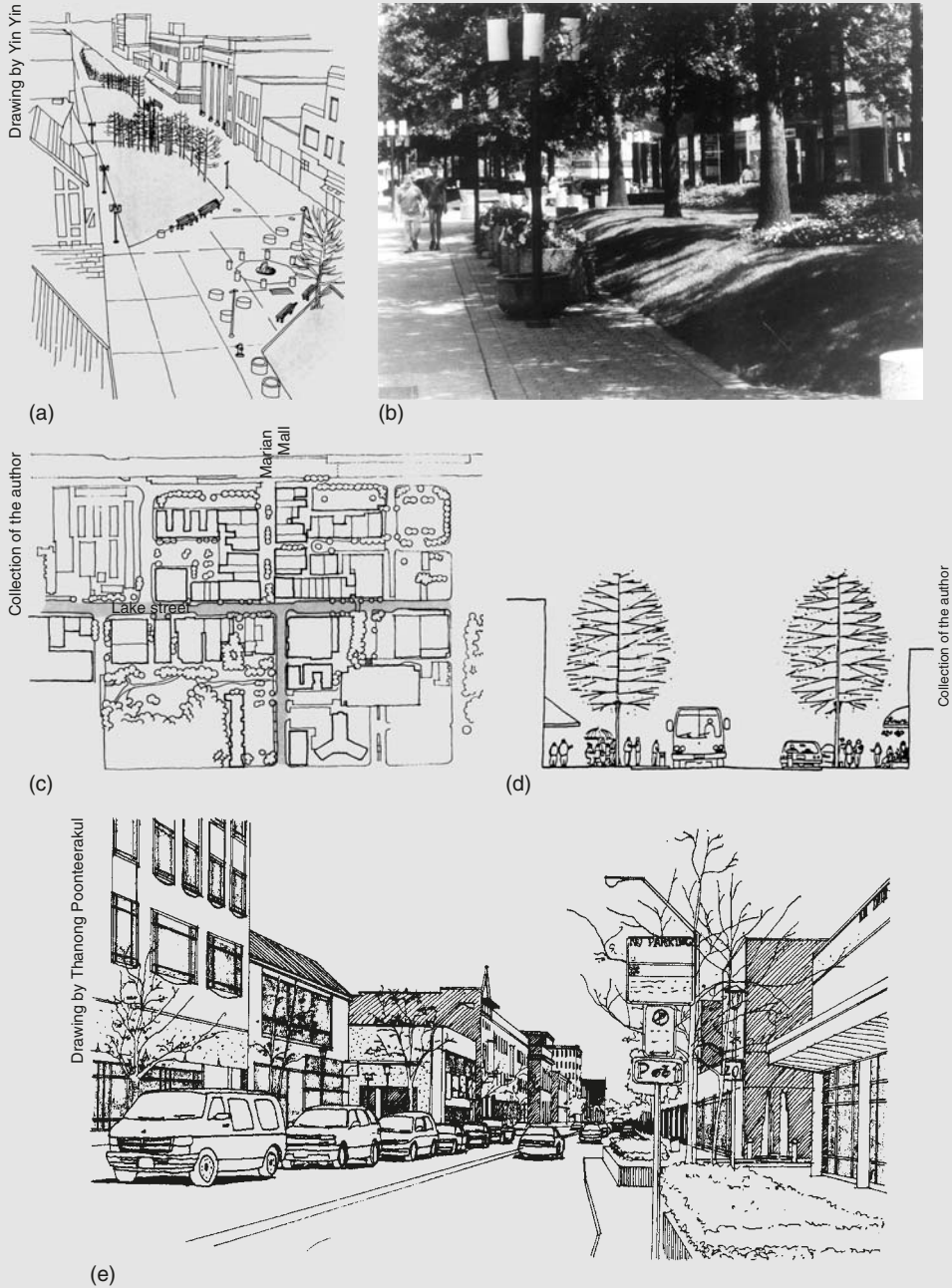
Figure 5.6 Oak Park Center Mall. (a) A sketch of Lake Street pedestrianized, (b) a view of the Mall in 1988, (c) the master plan for returning Lake Street to vehicular traffic, (d) a cross-section of Lake Street as proposed in the master plan and (e) Lake Street in 2004.
