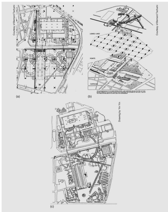
**Figure 5.17** The Parc de la Villette, Paris. (a) Tschumi and team's competition winning entry, (b) the design deconstructed and (c) the park as built.
