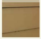
Available in panels and planks, fiber cement is a combination of cement, sand, wood fiber, and sometimes, clay. Like all products containing cement, fiber cement requires large amounts of energy to produce, which contributes to carbon dioxide emissions and global warming. Additionally, the wood fiber used in fiber cement is usually imported. Conventionally used for home siding, fiber cement is growing increasingly popular for fences.
