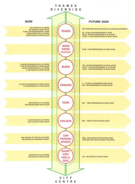
The diagram describes the concept of an 'interchange spine' stretching from a city centre location to the River Thames within which different modes of transport coincide, enabling changes between modes while minimising the 'interchange penalty' – the time it takes to change between modes. The diagram indicates current and future potential movements or flows as 'performance standards'.
