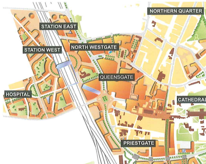
Annotation on top of a drawing obscures information and can look clumsy
