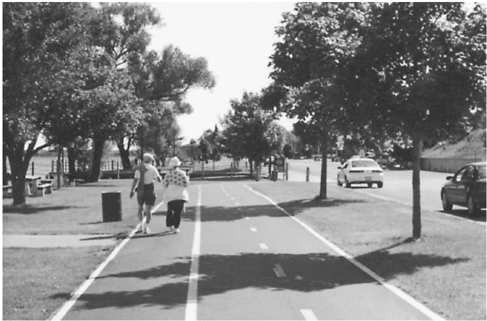
Figure 4.42 Photograph of separate travel lanes.
