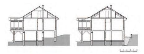
**Figure 4.** Basement (a) before, and (b) after restoration. Photo Milijana Okilj.
