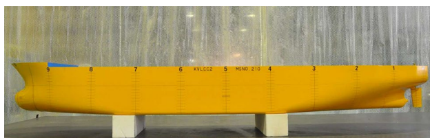
Fig. 2 Side profile of a KVLCC2 model
