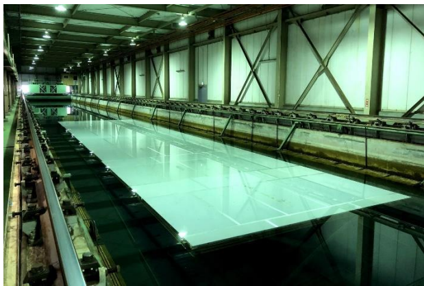
Figure 1. Photograph of the Hiroshima University towing tank equipped with a false bottom
