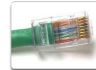
Good connector - Wires are untwisted to the extent necessary to attach the connector.
