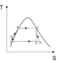
$$Isentropic efficiency = \frac{h_1 - h_{2'}}{h_1 - h_2} = \frac{W_{12'}}{W_{12}}$$
