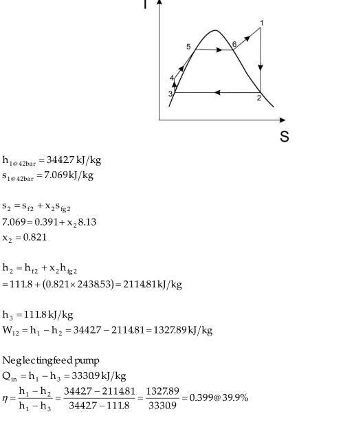
The thermal efficiency has increase due to superheating and improvement in SCC
