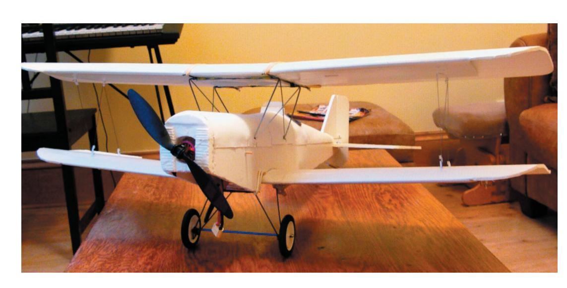
Propshaft height with a standard Flite Test power pod is correct for a 'low propshaft' version of the SE5a. Include a few degrees of down and side thrust. A 'correct scale' 11 inch prop will be very close to the ground; fine for tarmac or dirt,
