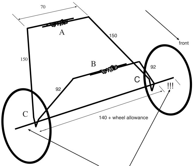
Depending on width of wheel used, allow extra at each end of axle for wheel width and collet/glue blob to attach wheel. 85mm wheel is scale.
