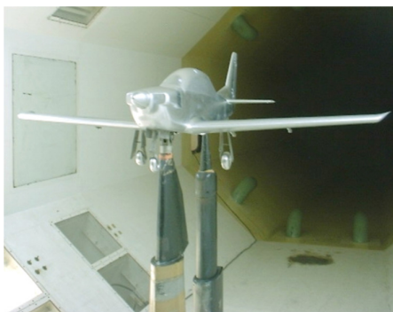
Fig. 2. TAM mounted on the TEM support in the T-35 wind tunnel test section [2]
