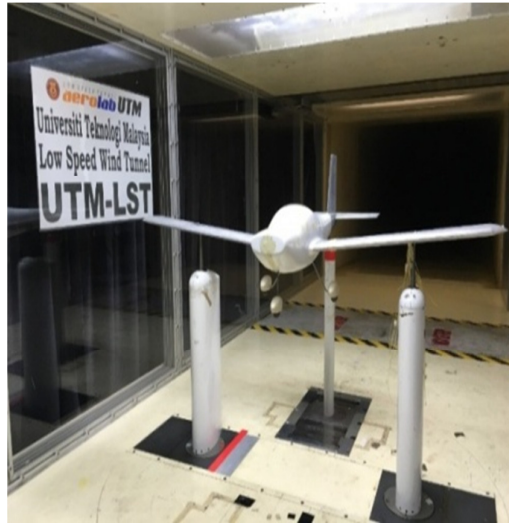
Fig. 5. Installation of UTM-LST light for clean wing configurations
