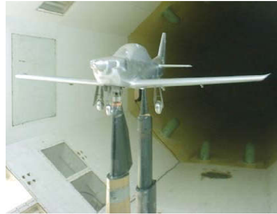
Fig. 2. The TAM mounted on the TEM support in the T-35 wind tunnel test section [2]
