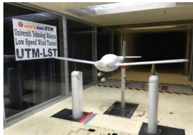
Fig. 5. The installation of UTM-LST light for clean wing configurations
