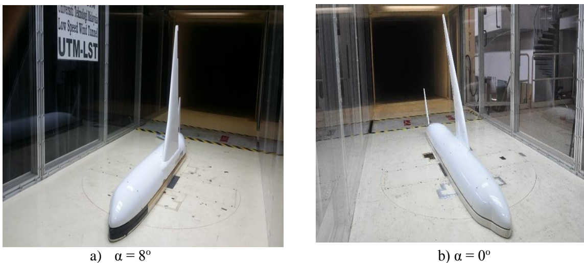
Figure 4. The installation of half-span model in UTM-LST
