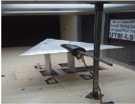
Figure 4: The installation of UTM VFE-2 model at \alpha=5^\circ
