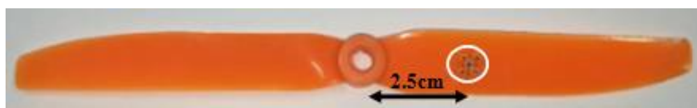
Figure 3.8: GWS slow flyer 8' x 4' propeller location of mass 3
