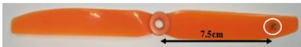
Figure 3.6: GWS slow flyer 8' x 4' propeller location of mass 1
