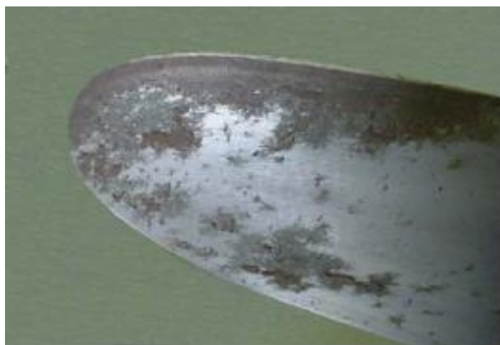
Figure 2.5: Polished Blade Surface Corrosion
