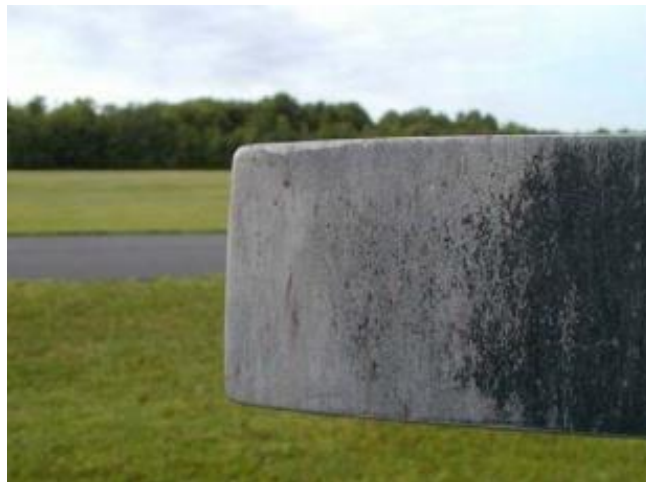
Figure 2.9: Erosion on a Metal Blade
