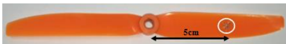
Figure 3.7: GWS slow flyer 8' x 4' propeller location of mass 2
