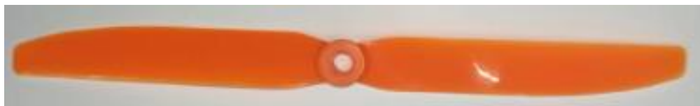
Figure 3.5: GWS slow flyer 8' x 4' propeller control
