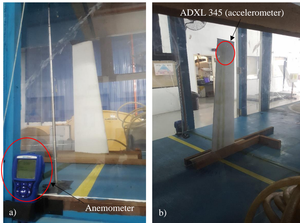
Figure 3.5 Setup for wing inside the wind tunnel. a) front view, b) rear view
