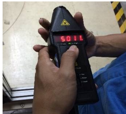
Fig 4. Tachometer to measure the propeller speed
