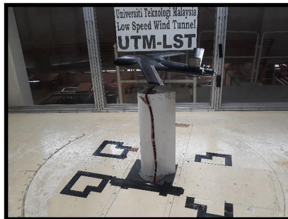
Figure 3.8: Wind tunnel testing for yaw angle
