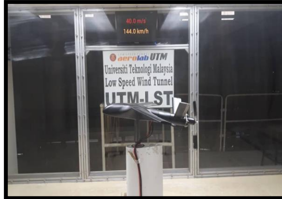
Figure 3.7: wind tunnel testing for pitch angle
