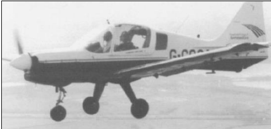
Figure 2.5: Nose powerplant – Scottish Aviation Bulldog (Source as adapted from book Aircraft conceptual design synthesis by DENIS HOWE)
