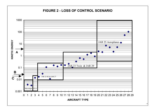
Kinetic Energy (as plotted) = (Mass (kg) X Velocity  $(kt)^2$ ) / 10<sup>9</sup>
