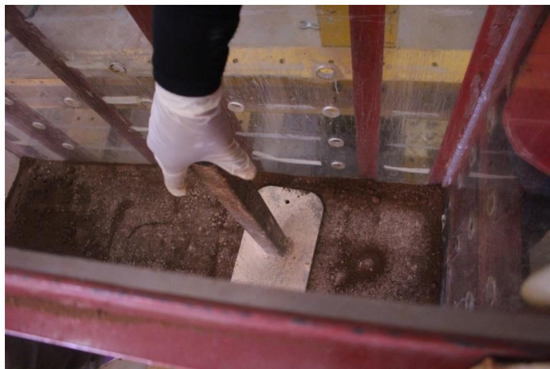
Figure 3.26: Manual compaction of the ground model using a hand tool
