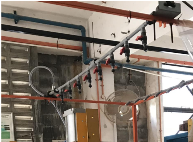
Figure 3.12: Rainfall flow nozzles each with its regulators
