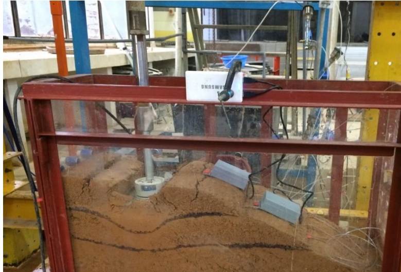
Figure 3.21: The two AWAM devices on top of a ground model being powered by a Power Bank clamped to the testing chamber during loading stages
