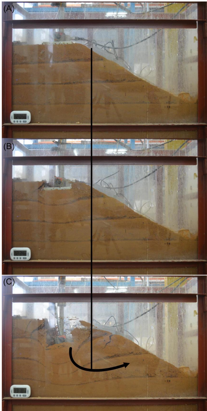
Figure 5.14: Slope deformation of the ground model for Case B; (A) initial state (B) significant AWAM device reading and (C) final condition after maximum loading
