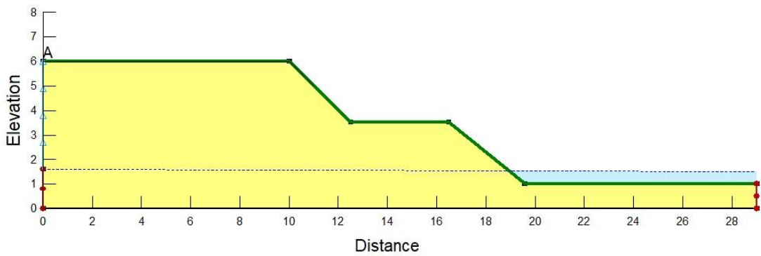
Figure 7.36: Site CICT geometry and boundary conditions
