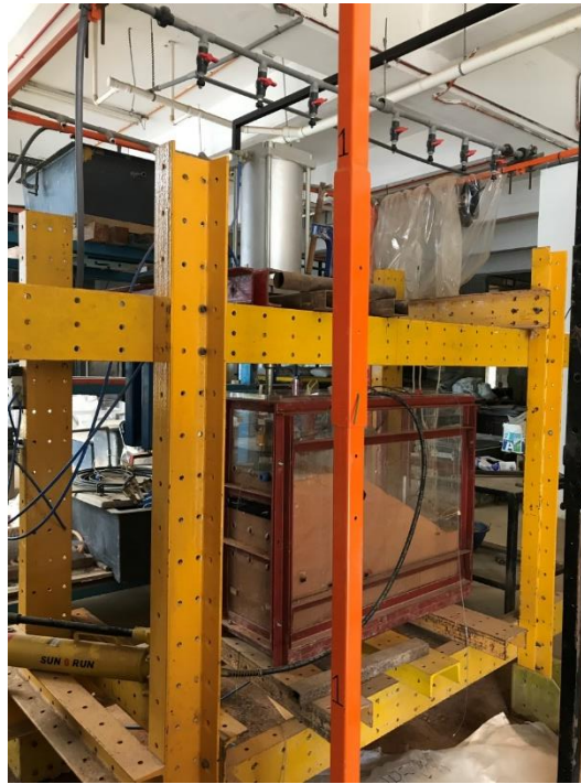
Figure 3.6: Loading frame housing a testing chamber in physical modelling tests
