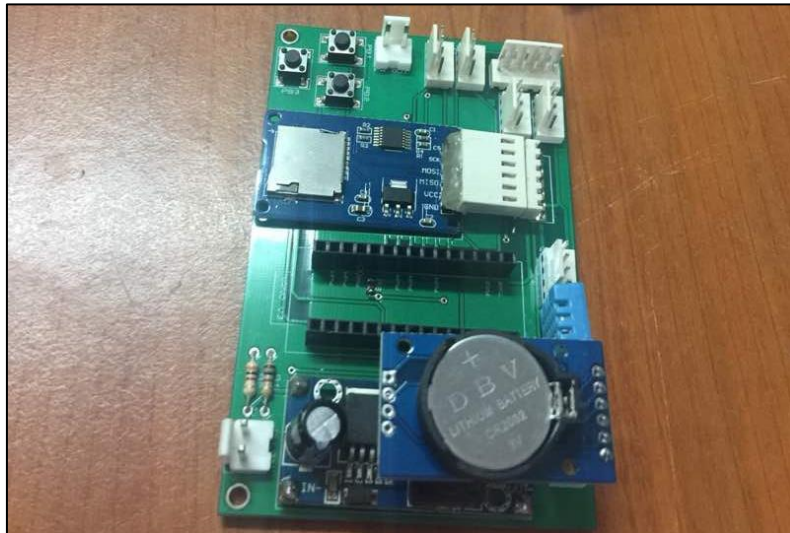
Figure 7.22: The on-board data and time management board for the date and time specifications of the AWAM system
