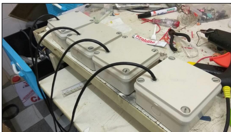
Figure 7.10: Enclosure box of the casing for the sensors of the AWAM system
