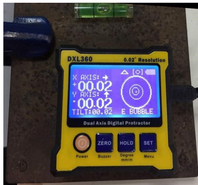
Figure 4.3: Dual axis digital protractor model DXL360 manufactured by Shenzhen Capital Electronics Co., Ltd. checked for flat surface readings using a bubble level
