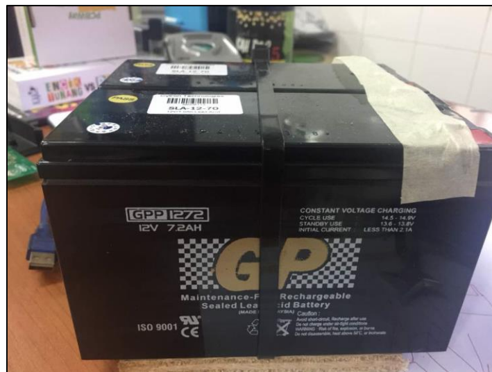
Figure 7.16: GP Seal Lead Acid (SLA) rechargeable battery used in the power capacity of the AWAM system
