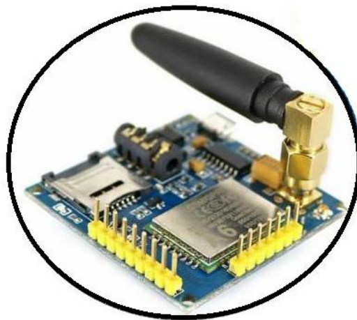
Figure 7.20: Wireless transmitter module manufactured by Arduino Uno for the data transmitting apparatus of the AWAM system
