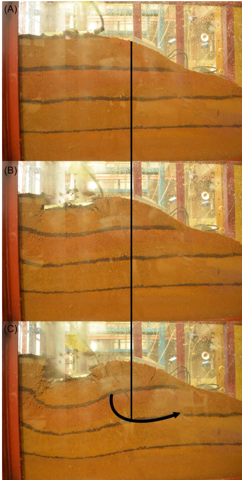
Figure 5.13: Slope deformation of the ground model for Case A; (A) initial state (B) significant AWAM device reading and (C) final condition after maximum loading
