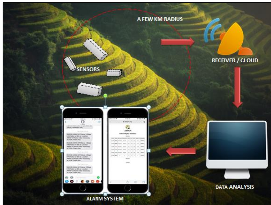
Figure 7.2: Diagram Process of AWAM System
