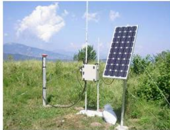
Figure 2.47: Solar powered GPS rover (Bertacchini et al., 2009)
