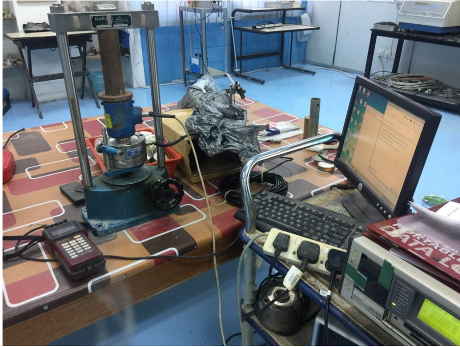
Figure 3.17: Calibration of load cell commencing in the UTM laboratory
