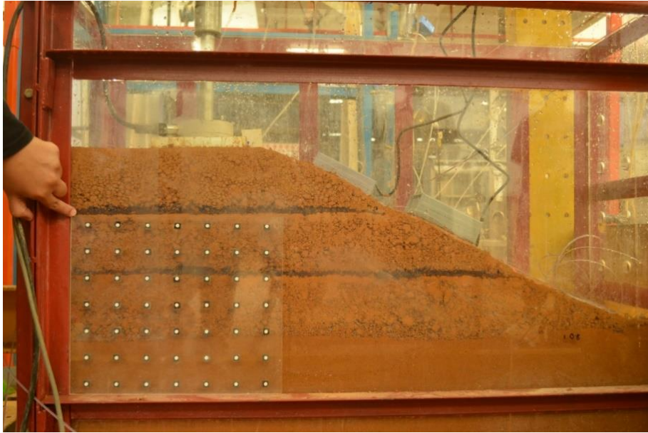
Figure 3.13: Target marker displayed in front of a ground model
