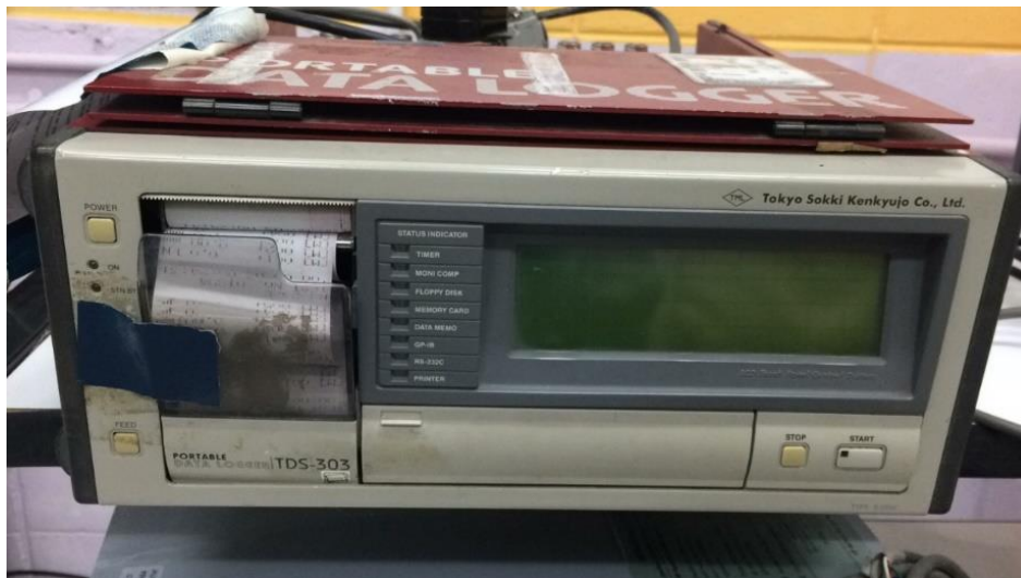
Figure 3.16: Portable data logger TML TDS-303 for loading stage data acquisition
