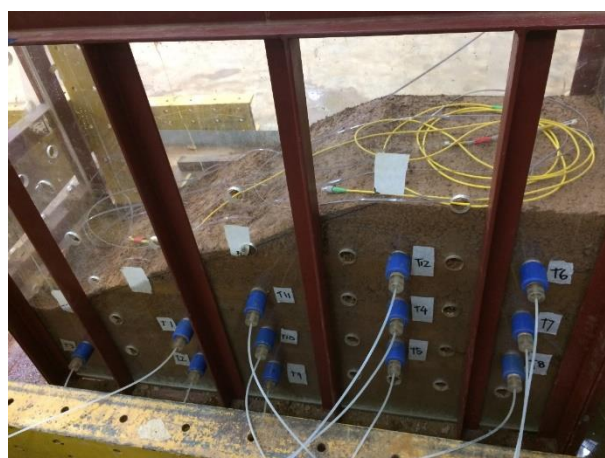
Figure 3.30: 12 units of tensiometer installation into the ground model
