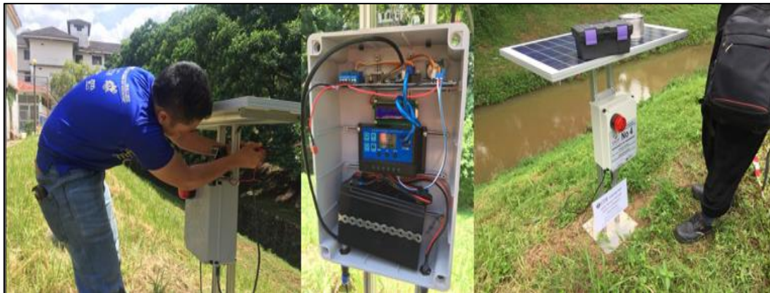
Figure 7.58: Setup of the AWAM system on site
