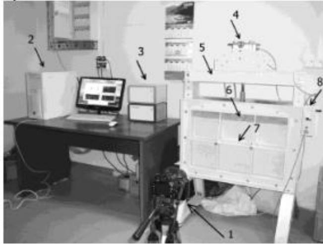
Figure 2.77: Automated foundation test set-up: 1- camera, 2- PC, 3- signal transmission unit, 4- pneumatic loading unit, 5- support beam, 6- load test plate with rod, 7- plexiglass wall with stiffener, 8- pressure control unit (Boldyrev et al., 2012)
