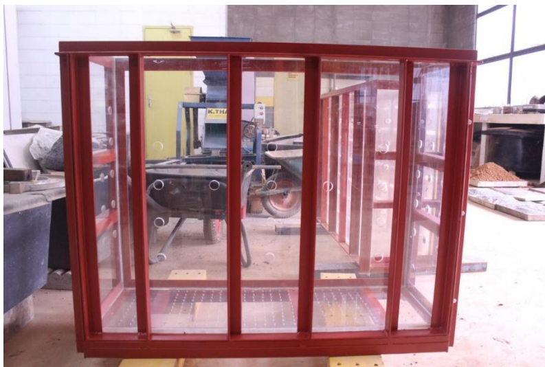
Figure 3.8: Tensiometer holes on the other side of the testing chamber
