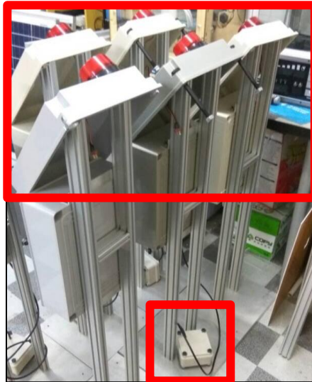
Figure 7.23: The casing of the power station and sensor casings assembled with tightening screw caps to ensure onboard systems are protected.
