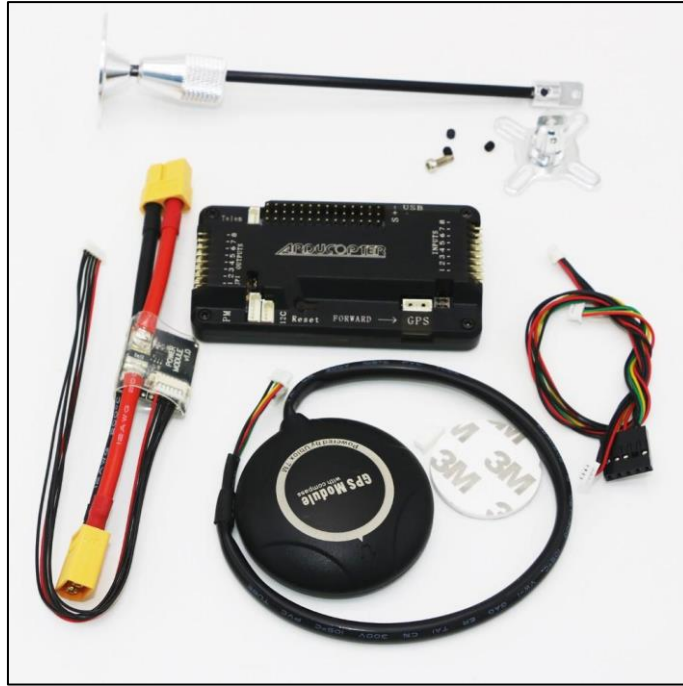
Figure 7.25: ArduPilot Mega (APM) flight controller used as the sensor mechanism in the AWAM system
