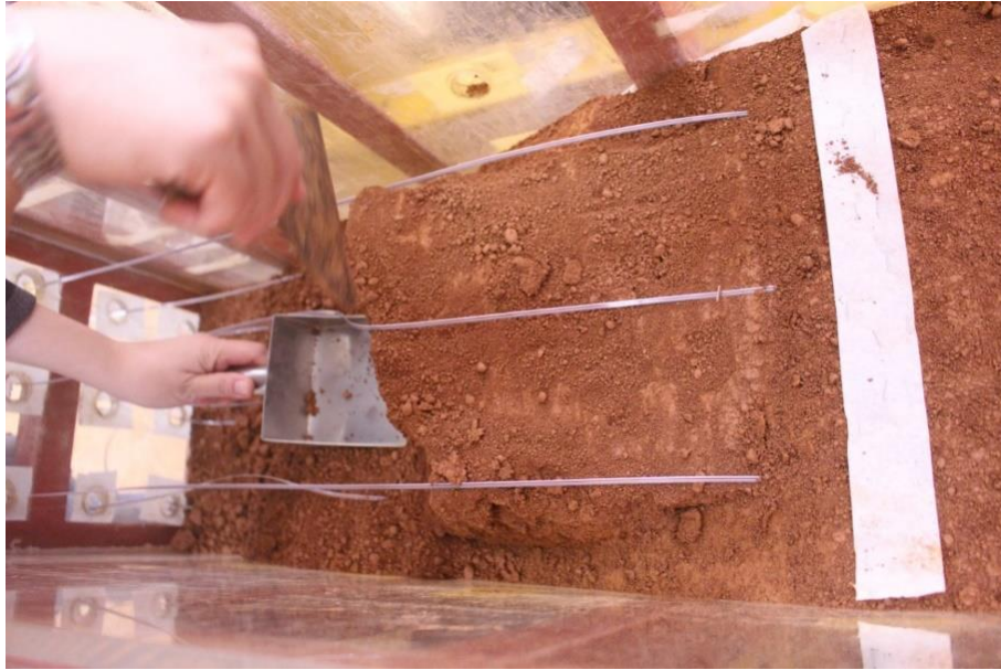
Figure 3.28: Reshaping the ground model onto its intended shape with hand tools
