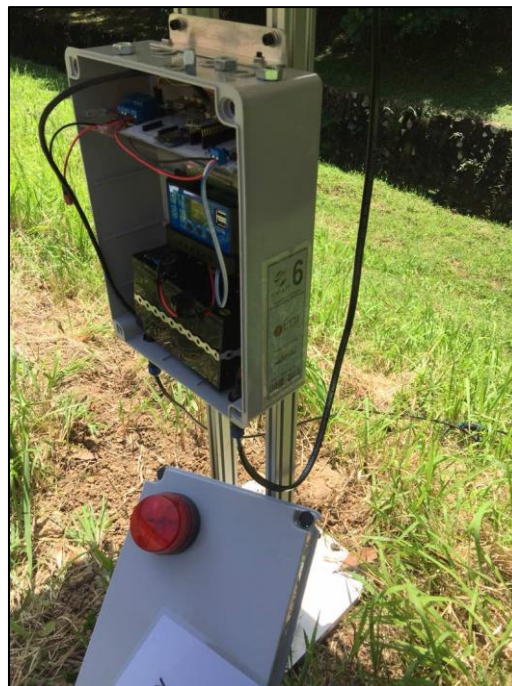
Figure 7.9: The overview of the waterproof enclosure box of the AWAM system in site conditions
