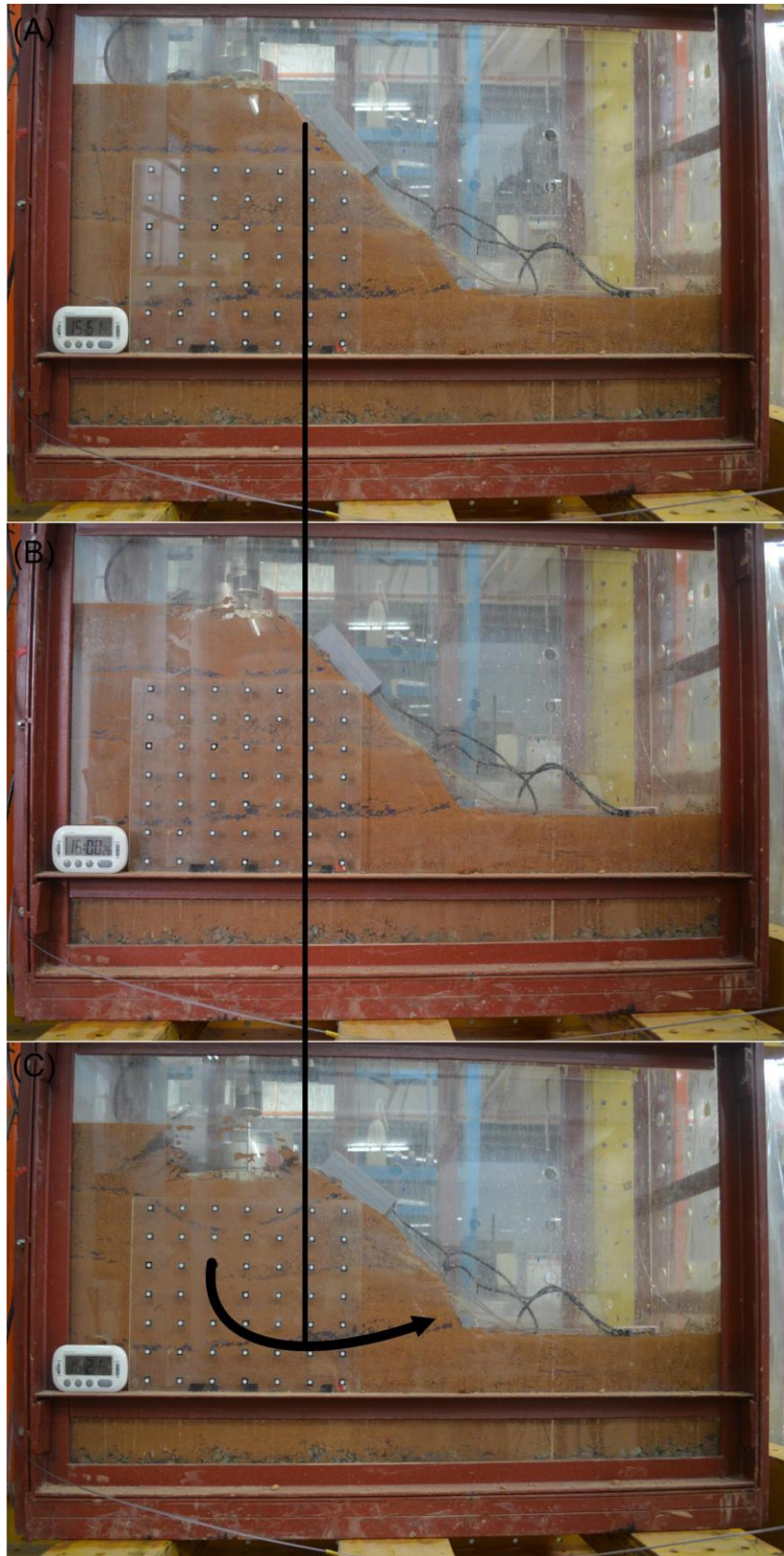
Figure 5.17: Slope deformation of the ground model for Case E; (A) initial state (B) significant AWAM device reading and (C) final condition after maximum loading
