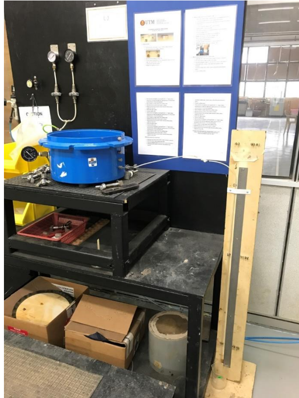
Figure 3.5: Pressure plate extractor setup in UTM
