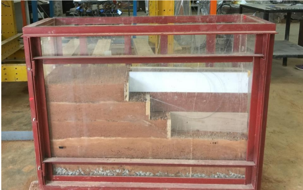
Figure 3.27: The compaction of the ground model being modelled into 5 layers and shaped with formwork whilst the first layer being layered with 50 mm gravel.
