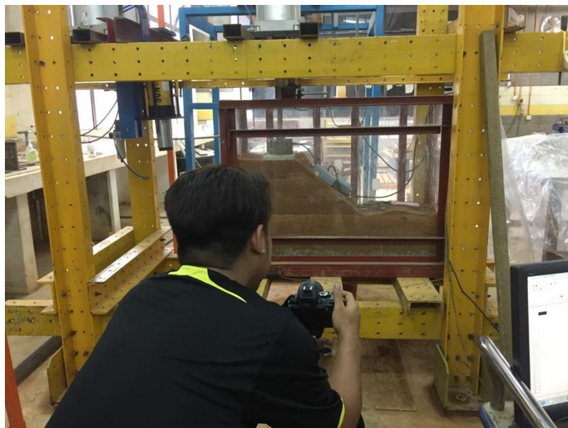
Figure 3.32: Camera Setup for PIV data acquisition
