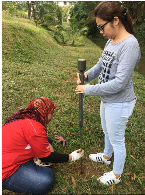
Figure 7.32: Mackintosh Probe test on site of the AWAM system prepared by research assistants
