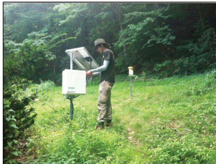
Figure 7.4: United States Geological Survey (USGS) open-canopy rain gauge on-site (Reilly et al, 2017)
