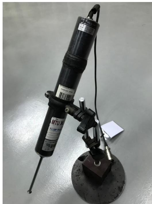
Figure 3.14: LVDT used to measure displacement units equipped with a magnet coupler
