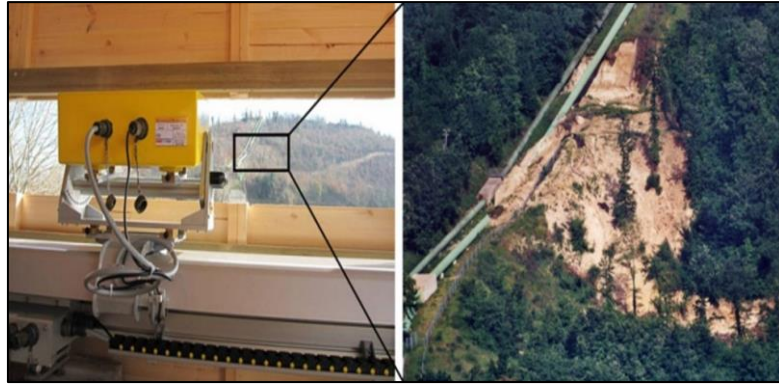
Figure 2.42: Monitoring System GBInSAR of the Site (Bozzano et al., 2010).
