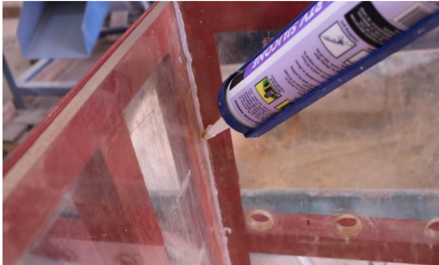
Figure 3.25: Filling the gaps between the testing chamber acrylic sides with silicone rubber
