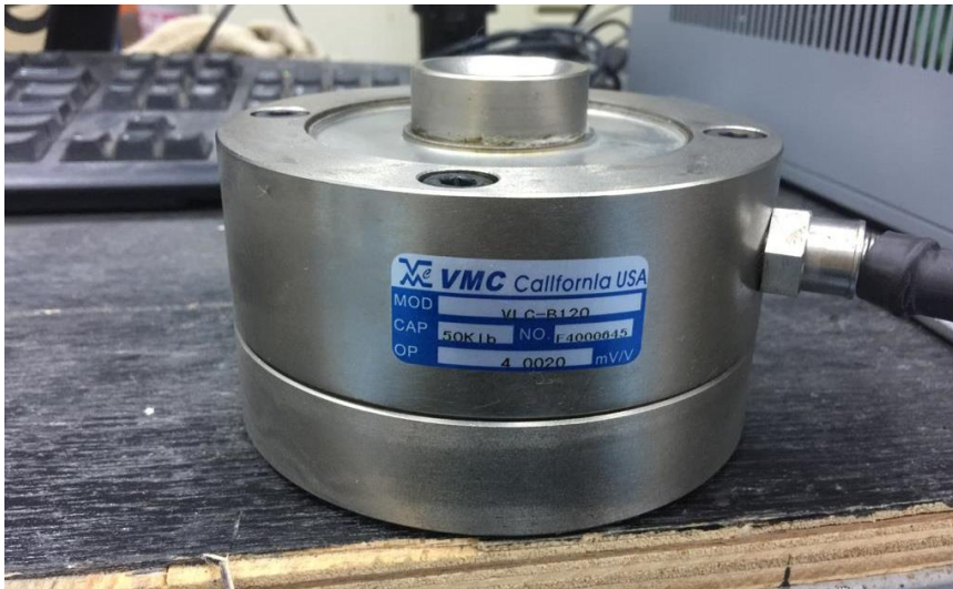
Figure 3.15: Load cell transducer made by VMC California USA used in the study
