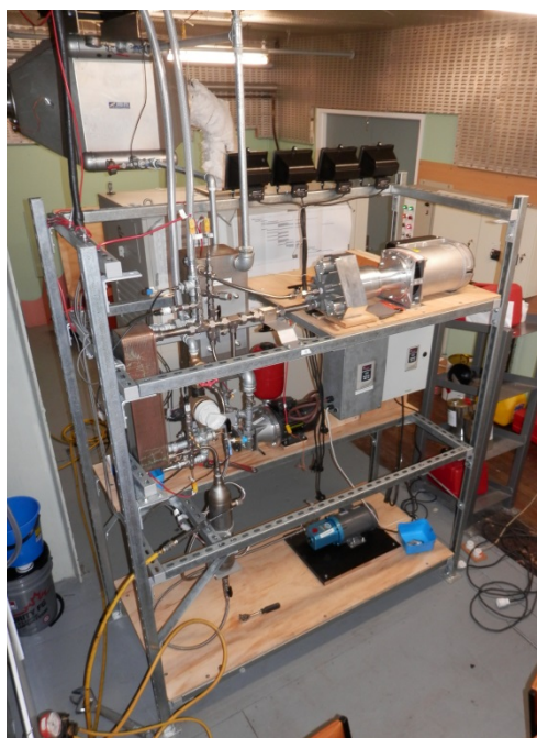
Figure 14 - ORC-B ready for testing
