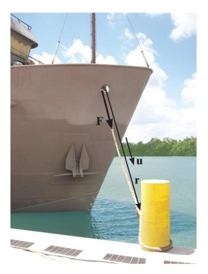
This ship's mooring line, connected to the bow, can be represented as a Cartesian vector.
