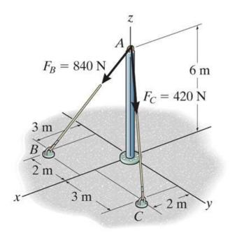
As per the figure, when relating A to C, we will have to go 2 m in the xdirection, 3 m in the y-direction, and -6 m in the z-direction. Hence,
