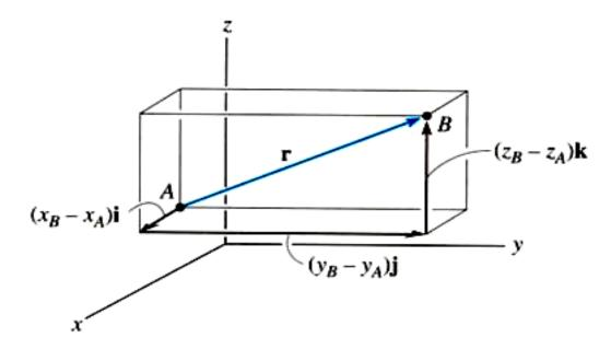
The position vector <u>directed from A to B</u>,  $r_{AB}$ , is defined as  $r_{AB} = \{(X_B - X_A)i + (Y_B - Y_A)j + (Z_B - Z_A)k\}m$ Please note that B is the ending point and A is the starting point. <u>ALWAYS subtract the "tail" coordinates from the "tip"</u> coordinates!
