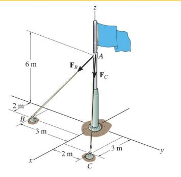
**Given:** Two forces are acting on a flag pole as shown in the figure.  $F_B = 560 \text{ N}$ and  $F_C = 700 \text{ N}$
