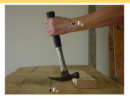
Carpenters often use a hammer in this way to pull a stubborn nail. Through what sort of action does the force  $F_H$  at the handle pull the nail? How can you mathematically model the effect of force  $F_H$  at point O?
