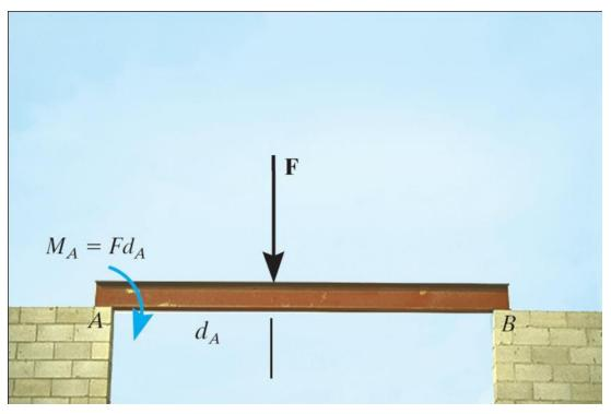
Beams are often used to bridge gaps in walls. We have to know what the effect of the force on the beam will have on the supports of the beam.
